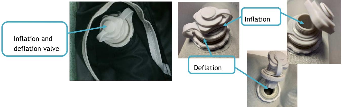
Given that the valves are connected to each other, it will not be possible to inflate the structure correctly if one of the stoppers is open.
